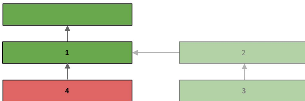
Figure 5.16: Illustration of selfish mining. This shows one of several possible ways in which the attack could play out. (1) Block chain before attack. (2) Attacker mines a block, withholds it, starts mining on top of it. (3) Attacker gets lucky, finds a second block before the rest of the network, continues to withhold blocks. (4) Non-attacker finds a block and broadcasts it. In response, the attacker broadcasts both his blocks, orphaning the red block and wasting the mining power that went into finding it.
