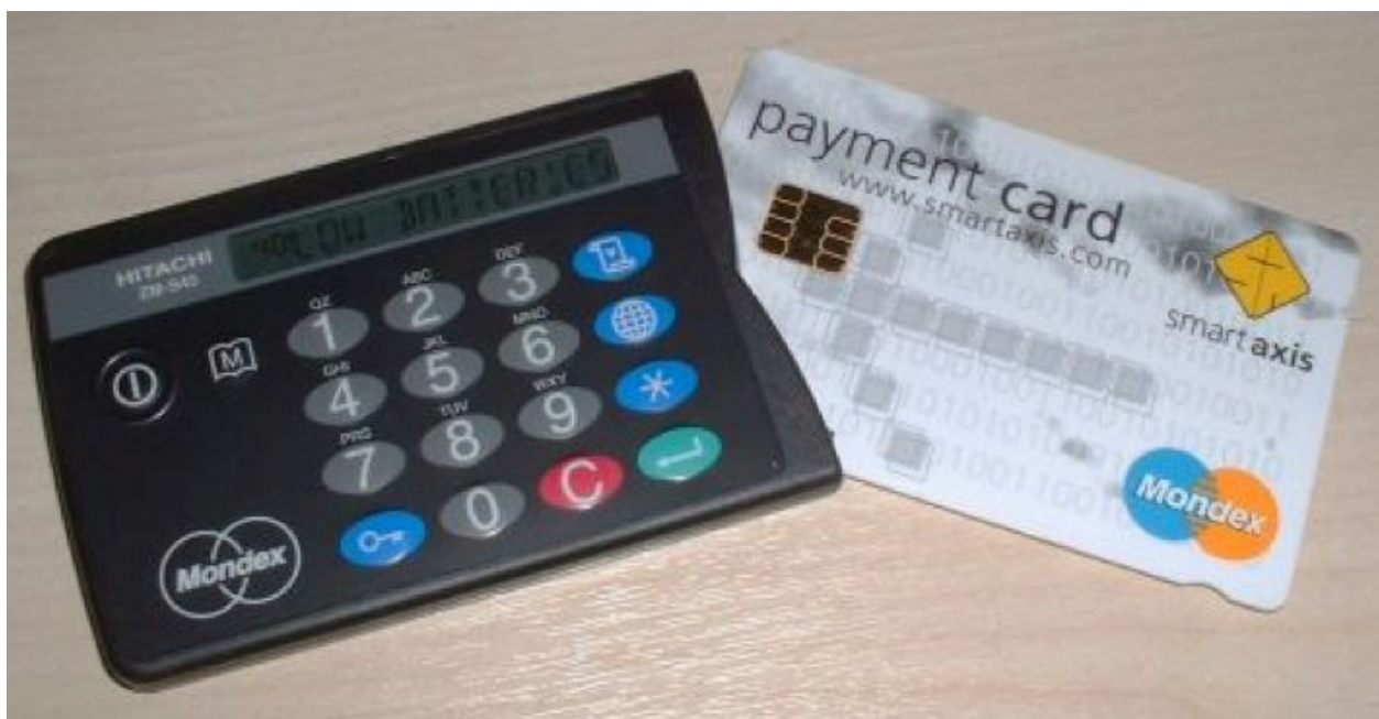
Figure 3: Mondex system, showing user card and wallet.
