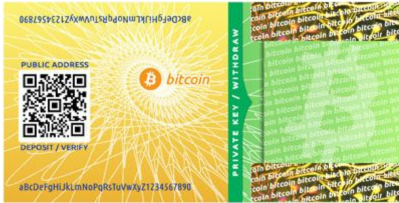
Figure 4.3: A Bitcoin paper wallet with the public key encoded both as a 2D barcode and in base 58 notation. Observe that the private key is behind a tamper-evident seal.
