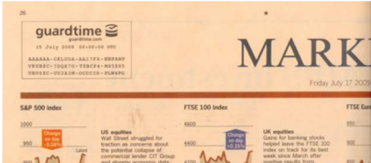
Figure 9.2: A timestamping service (GuardTime) that publishes hashes in a daily newspaper rather than the Bitcoin block chain. Customers of the company can pay to have their data included in the timestamp. Recall from Chapter 1 that we can use Merkle trees to encapsulate many pieces of data in a single hash and still efficiently prove that any one of those pieces of data is included in the hash.
