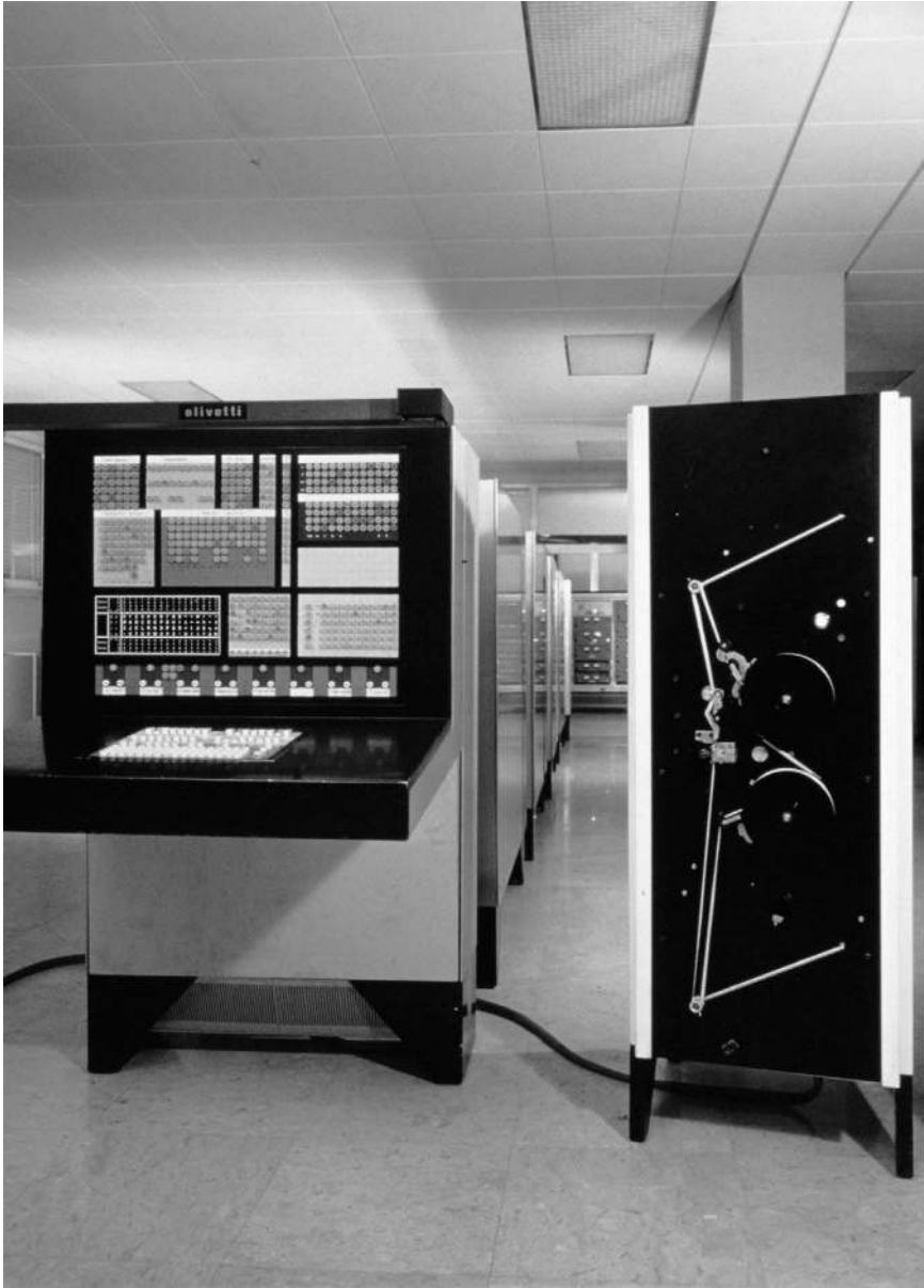
Figure 3.3 The central control console with the photoelectric perforated band reading unit on the right. (Associazione Archivio Storico Olivetti, Ivrea, Italy).
