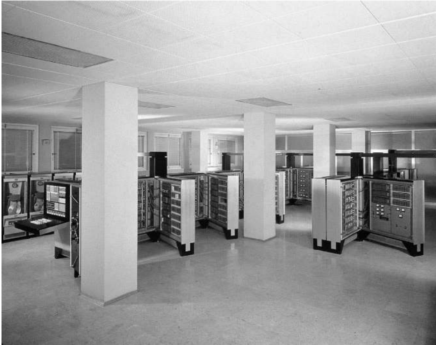
Figure 3.2 The Elea 9003 mainframe computer is a system designed by Ettore Sottsass comprised of modules of standard metal cabinets connected by a series of overhead busways. (Associazione Archivio Storico Olivetti, Ivrea, Italy).
