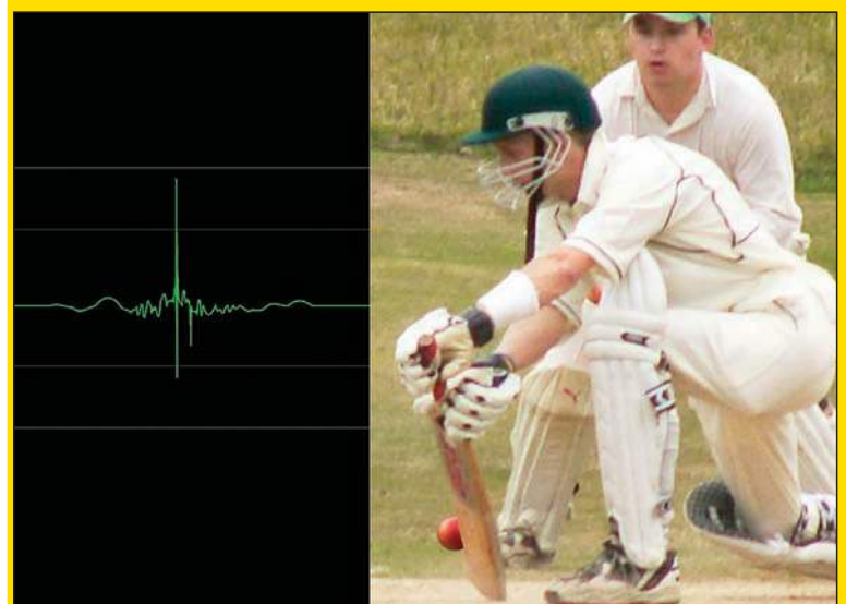
The Snickometer displays a high peak on the sound graph to show contact with the bat. These peaks are distinctly different from other sounds, such as that of the bat hitting the pad.
